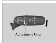
When you push the lever down to **AUTO**, the windshield wipers sweep once, and go into the automatic mode.
