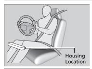
Housing Location The knee airbag for the driver and the one for the front passenger are housed under the steering column and the glove box respectively.
