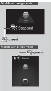
Your vehicle also stops, automatically. The **Stopped** message appears on the gauge. When the vehicle ahead of you starts again, the vehicle icon on the gauge blinks. If you press the **RES/+/SET/-** switch up or down, or depress the accelerator pedal, ACC with Low Speed Follow operates again within the prior set speed.
