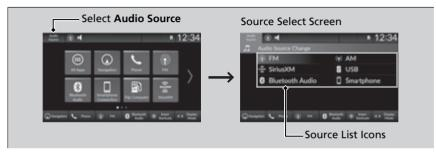
Select **Audio Source** on the header area, then select an icon on the source list to switch the audio source.
