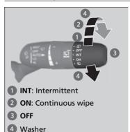
The rear wiper and washer can be used when the power mode is in ON.
