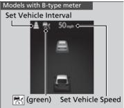
When ACC with Low Speed Follow starts operating, the vehicle icon, interval bars and set speed appear on the gauge.
