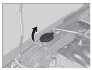
If the level is low, fill the washer reservoir.
