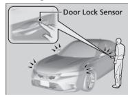
Touch the door lock sensor on the front door or press the lock button on the hatch.
