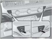
Press the seat heater button: Once - The HI setting (three indicators on) Twice - The MID setting (two indicators on) Three times - The LO setting (one indicator on)
