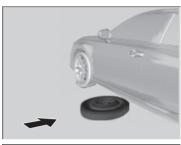
**6.** Place the compact spare tire (wheel side up) under the vehicle body, near the tire that needs to be replaced.
