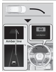
The front wide view camera behind the rearview mirror monitors left and right lane markings in white or yellow, the outer edge of the pavement (bordered by grass or gravel) or a detected oncoming vehicles.
