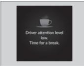
If one bar lights up, the **Driver attention level low. Time for a break.** message will appear, a beep will sound, and the steering wheel will vibrate.
