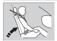
Adjust the driver's seat-back to a comfortable, upright position, leaving ample space between your chest and the airbag cover in the center of the steering wheel.
