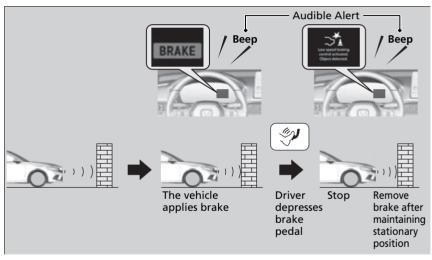
If the only rear sensors are turned off using the parking sensor system, the Low Speed Braking Control is not working when reversing.
