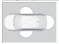
When you carry the keyless remote, you can lock/unlock the doors, fuel fill door and hatch. You can lock/unlock the doors, fuel fill door and hatch within a radius of about 32 inches (80 cm) of the outside door handle or hatch release button
