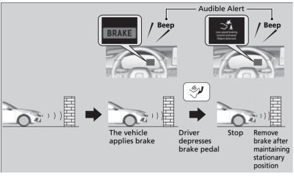
If the only rear sensors are turned off using the parking sensor system, the assistive braking is not working when reversing.
