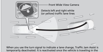
center of the lane and the system has detected the traffic lane lines.
