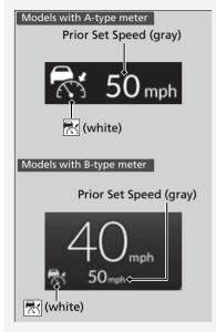
The set speed cannot be set or resumed when ACC with Low Speed Follow has been turned off using the button. Press the button to activate the system, then set the desired speed.
