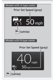
The set speed cannot be set or resumed when ACC has been turned off using the button. Press the button to activate the system, then set the desired speed.
