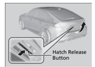
When all the doors are unlocked or press the hatch unlock button on the remote transmitter, the hatch is unlocked. Press the hatch release button and lift open the hatch.
