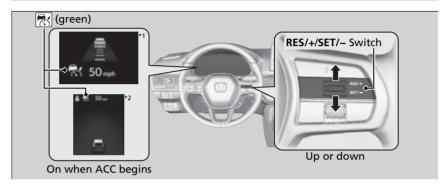
Take your foot off the pedal and press the **RES/+/SET/-** switch up or down when you reach the desired speed. The moment you release the button, the set speed is fixed, and ACC begins.
