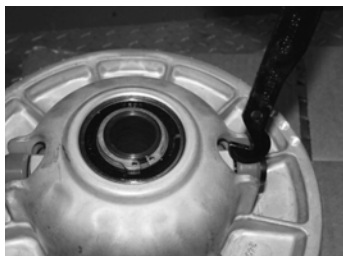
Insert hooked end of tool.
